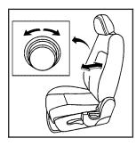
If your vehicle has this feature, the knob is located on the inboard side of the driver's seatback.
